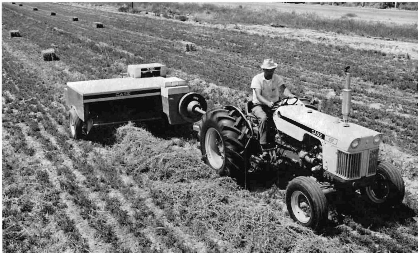
The most common method of haying in Wyoming is to swath the hay and bale it with string or wire ties and pick up the bales with front end loaders or with bale wagons.
