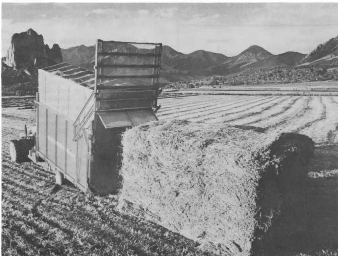
This Stakhand, powered by a 100 hp tractor, picks up windrowed hay, compresses it into 4-5 ton loaf-like stacks and unloads mechanically. Designed for loose hay handling, the new cost of this Stakhand and tractor is about $26,000.
