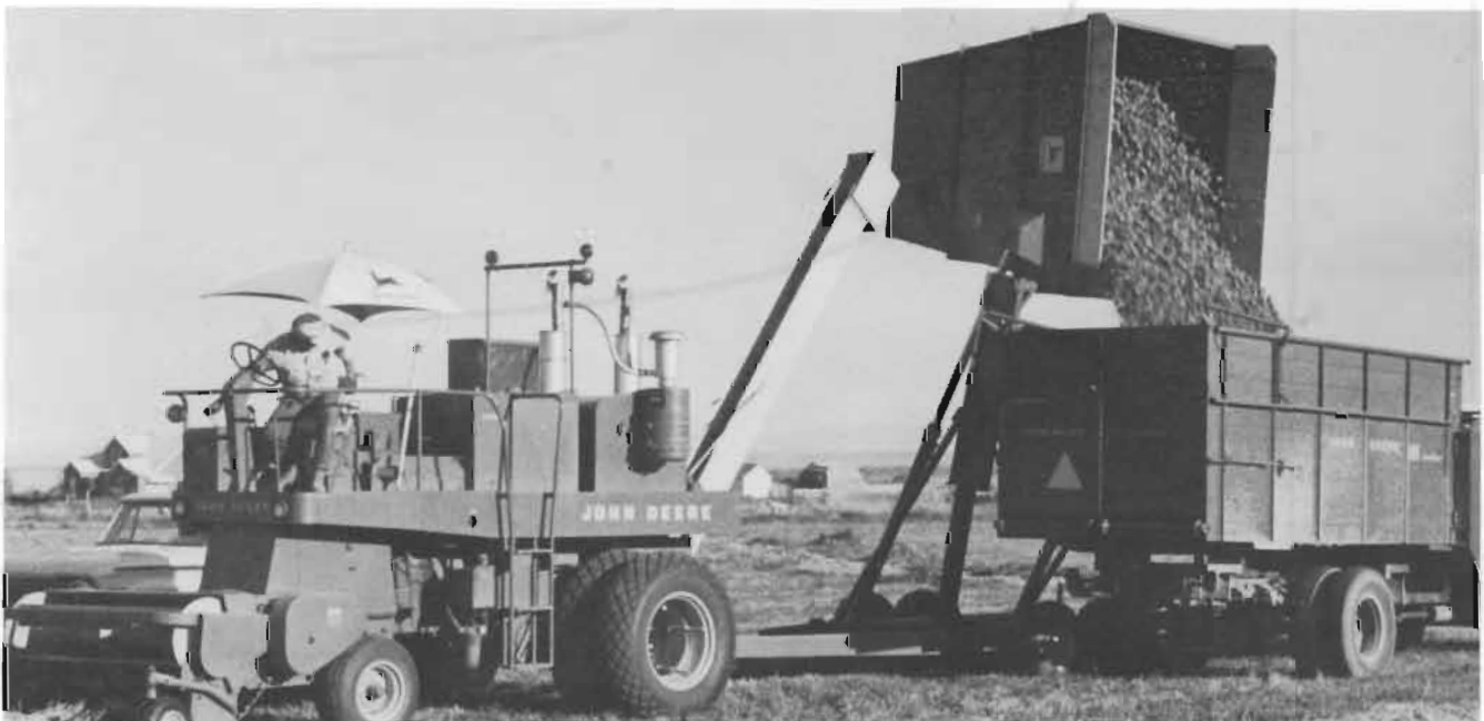
This self propelled mobile cubing unit requires an investment of about $40,000. In addition, a truck to haul cubes and another to haul water is needed. A ton of hay after being thoroughly dried in the windrow is sprayed with about 200 pounds of water as it is picked up. After grinding, the hay is forced through dies which result in cubes approximately 1\frac{1}{4} \times 1\frac{1}{4} \times 2\frac{1}{2} inches. The loaded cart is raised hydraulically and the cubes dumped into a truck.
