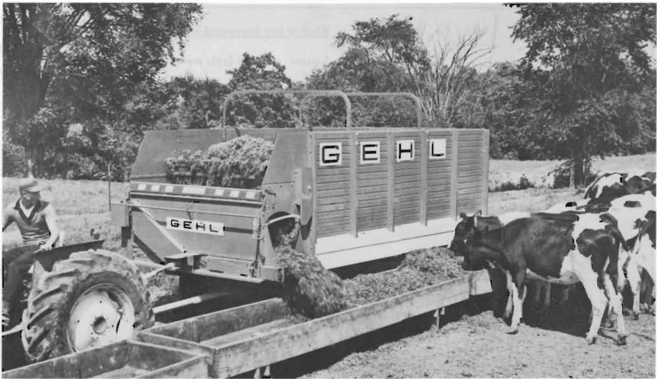
Haylage (hay wilted to about 50% moisture and then ensiled), placed in a feed mixer by a front end loader, is mechanically augered into feed bunks.
