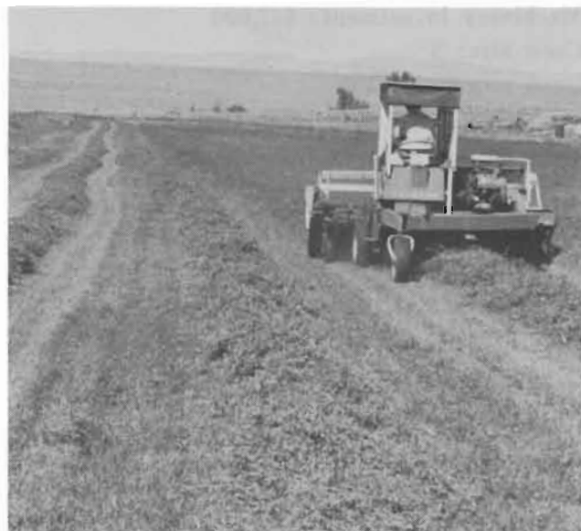
Most Wyoming hay is harvested with a swather which cuts and windrows. An attached conditioner flattens alfalfa and clover stems which permit faster drying. Conditioners are seldom used with native hay and never with ripening grain.
