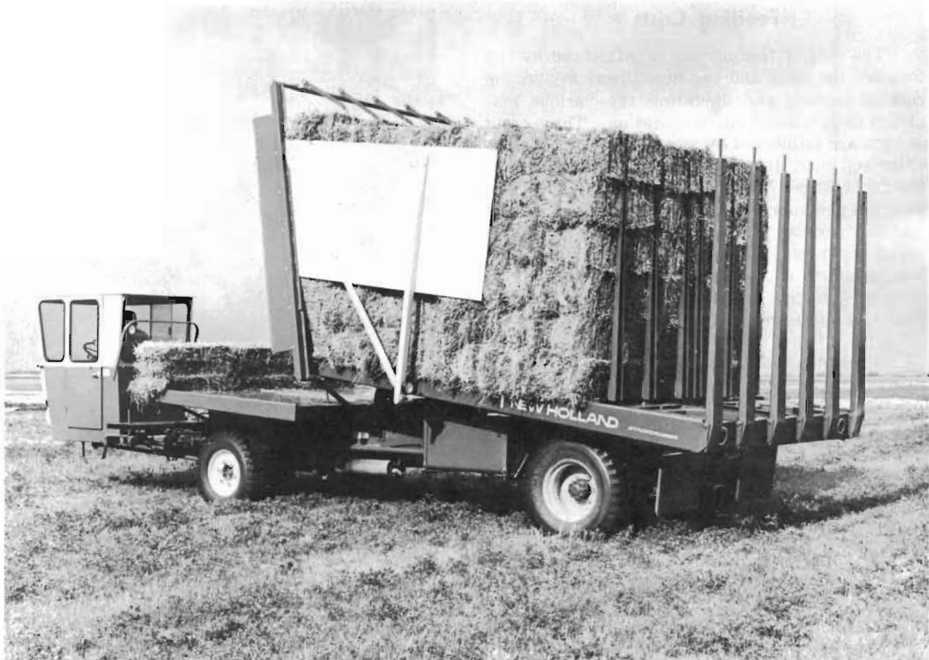
Tractor drawn or self-propelled bale wagons are popular because one man can stack 60-80 tons per day. The same load stacked at harvest time can be picked up in winter and hauled to the feeding area with this bale wagon.
