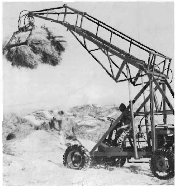
This grapple fork mounted on a self-propelled hydraulically operated stacker is a handy and efficient feeding arrangement. Two or three 800-pound forks full can be fed from a hay rack or the hay can be dribbled out to the livestock by shaking the fork.
